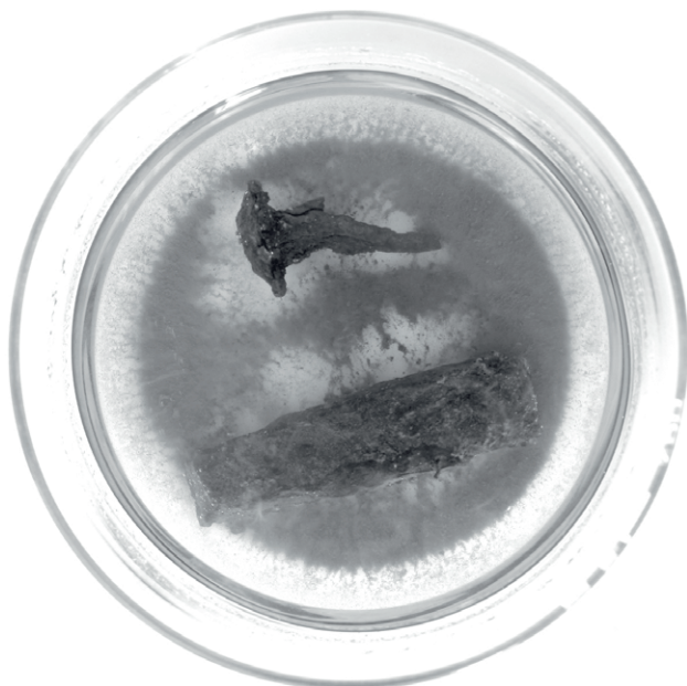
Figure 2: Immersion of archaeological iron objects in hydroxylamine. A reddish brown precipitate appeared on the bottom of the beaker after the first desalination bath
